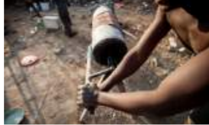
Fig 6: Wikus de Wet. 27 September, 2014. A teenager turns a customised gas cylinder filled with metal balls to crush the gold ore they extracted from under the ground.
